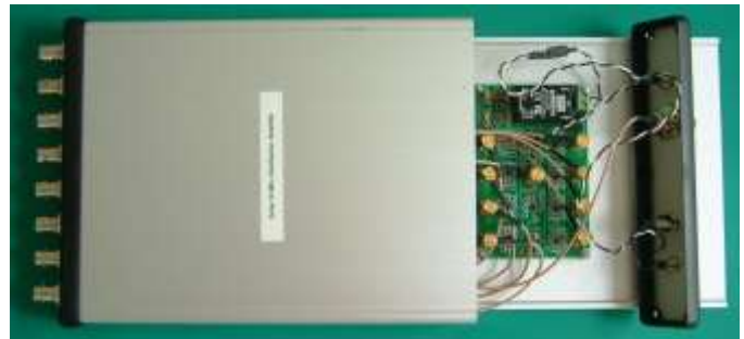
Figure 15. Interior View of Distribution Amp
